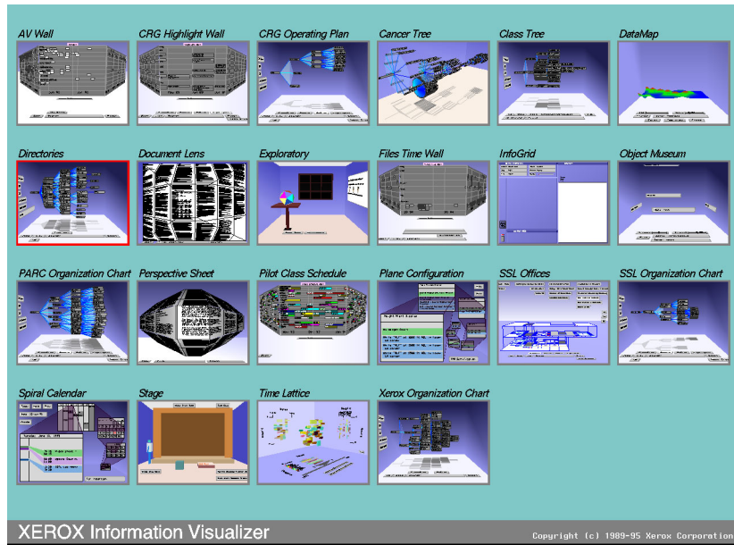
Figure 10: [Courtesy of Xerox PARC] The Rooms metaphor provides a set of distinct workspaces which can be used to collect applications, documents, and windows associated with a particular task or project. The overview allows finding and navigating between rooms. This Rooms overview shows a number of minaturized, but live, 3d workspaces containing Xerox PARC visualizations.
